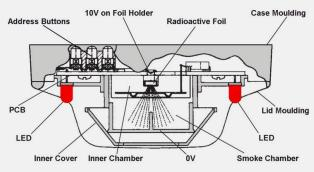
Figure 4 – Sectional View – Discovery Ionisation Smoke Chambe
