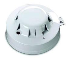
The Discovery Optical Detector has a white moulded polycarbonate case with wind-resistant smoke inlets. The indicator LEDs are colourless when the detector is in quiescent state and red in alarm. Within the case is a printed circuit board which, on one side, has the light-proof chamber with integral gauze surrounding the optical measuring system and, on the other, the signal processing and communications electronics.
