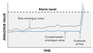
Figure 1 – Drift Compensation Graph
