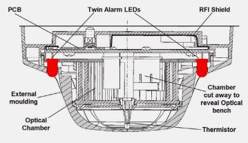
Figure 3 – Sectional View – Discovery Multisensor Detector
