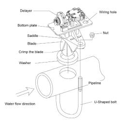
Figure 2 Installation Drawing
