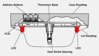
Figure 5 - Sectional View - Discovery Heat Detector
